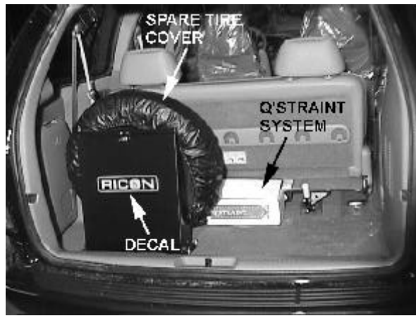
FIGURE [6-24]: CARGO AREA COMPONENTS
