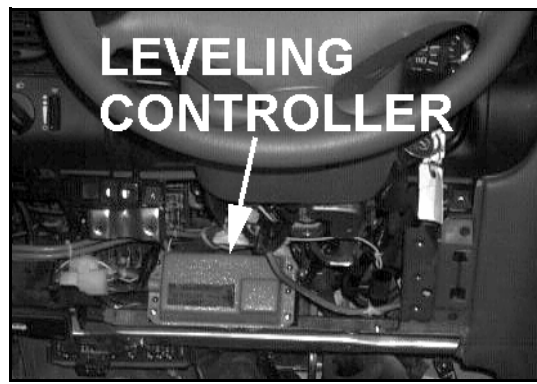
FIGURE [5-1]: LEVELING CONTROLLER LOCATION
