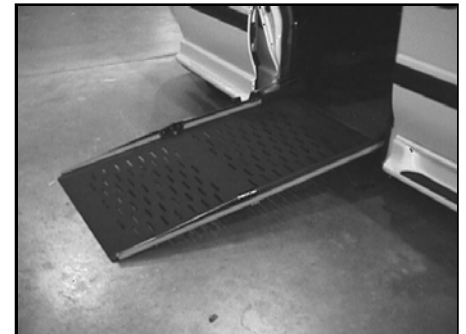
FIGURE 2-3: FOLDING RAMP DEPLOYED
