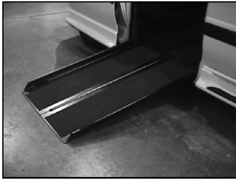
FIGURE 2-6: BACK-UP RAMP IN PLACE
