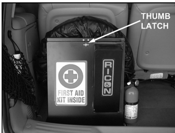
FIGURE 2-4: STORAGE BIN/SPARE TIRE MOUNT
