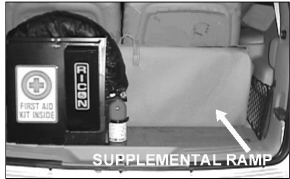
FIGURE 2-7: BACK-UP RAMP STORAGE LOCATION
