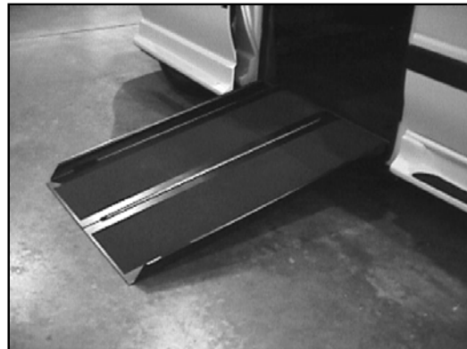
FIGURE 3-6: BACK-UP RAMP IN PLACE
