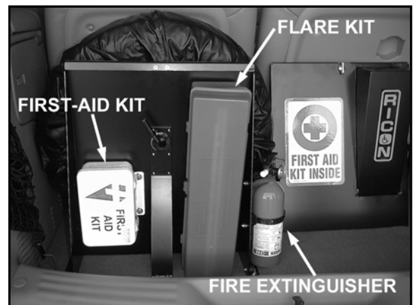
FIGURE 2-5: STORAGE BIN COMPONENTS
