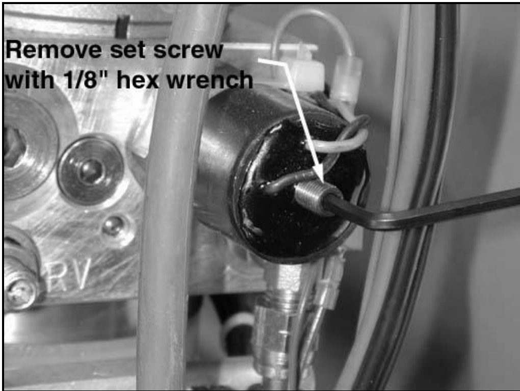
FIG [5]: PRESSURE SWITCH SET SCREW DETAIL
