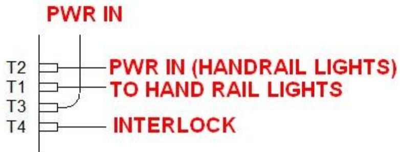
FIGURE 4: PREVIOUS TERMINAL ORIENTATION
