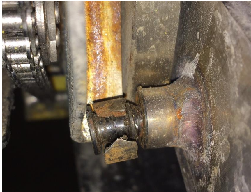
FIG. [3] EXAMPLE OF DAMAGED CAM FOLLOWER
