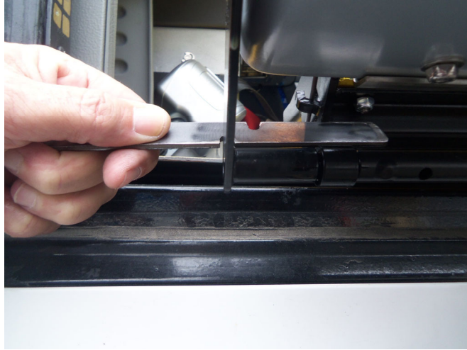
FIGURE 2-4: BRIDGEPLATE HEIGHT GAUGE TOOL SHOWN FOR CONFIG F9TF-DE019, F9TH-DE035
