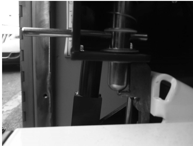
FIGURE 4-42B: VERIFY GAPS WITH TOOL P/N 55273
