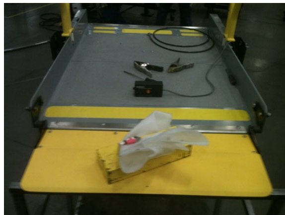
FIGURE 2-7. 25 LB. (11 KG) LOAD TEST (CENTER SIDE)
