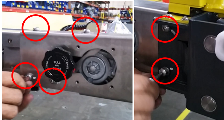
FIGURE 4-8: RIGHTHAND ROLLSTOP MAIN COVER BOLT LOCATIONS
