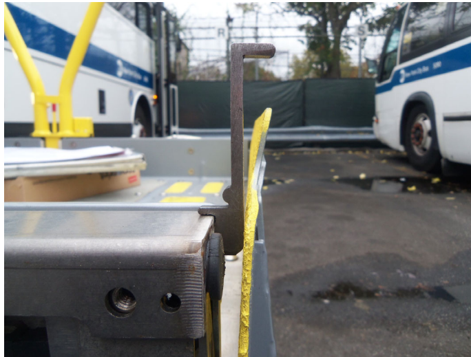
FIGURE 4-18: IN THIS ORIENTATION, GAGE TOOL (P/N 55273) WILL PREVENT LIFT FROM RISING
