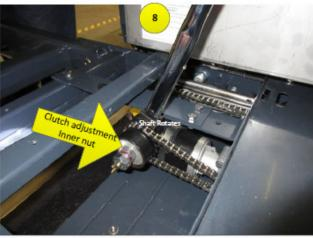
To adjust the torque setting on the clutch, either loosen(to reduce) or tighten (to increase) the inner nut against the clutch plate
