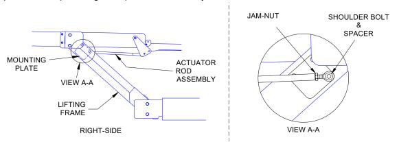
FIGURE 4-32: BRIDGEPLATE ACTUATOR ROD REMOVAL
