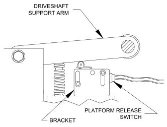
FIGURE 4-41: PLATFORM RELEASE SWITCH SETTING
