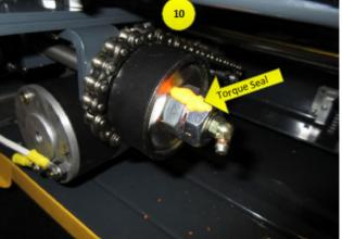
Apply torque seal across both nuts, once complete.
