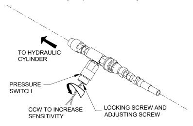
FIGURE 2-17: ANTI-STOW PRESSURE SWITCH
