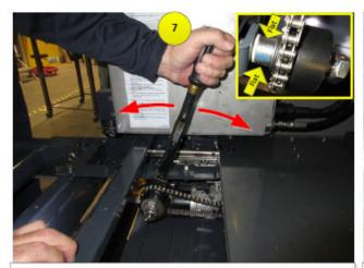
Using a 22mm clawfoot torqure wrench (which can measure up to a max. of 30ft.lbs).
