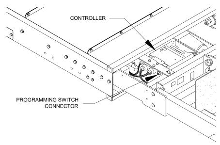
FIGURE 2-16: PROGRAMMING SWITCH CONNECTOR
