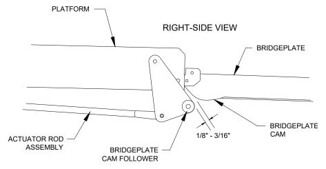
FIGURE 2-4: BRIDGEPLATE ADJUSTMENT
