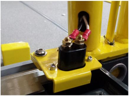
FIGURE 4-49: CONTACT SWITCH
