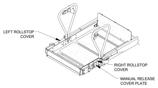
FIGURE 4-3: ACCESS COVERS FOR ROLLSTOP MECHANISM
