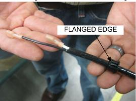
FIGURE 4-29. DISCONNECT BRIDGEPLATE SWITCH CONNECTORS
