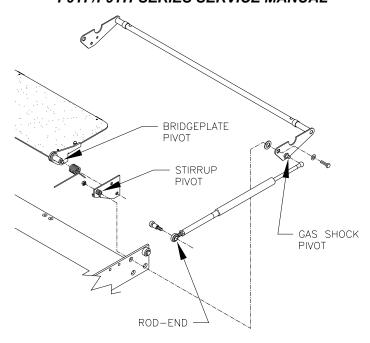
FIGURE 4-28: ACTUATOR ROD AND STIRRUP HARDWARE ASSEMBLY
