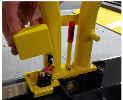
FIGURE 4-48: CONTACT SWITCH ENCLOSURE
