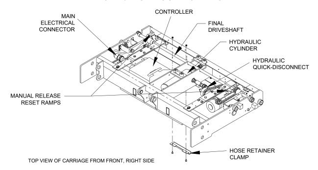
FIGURE 4-36: CARRIAGE COMPONENTS
