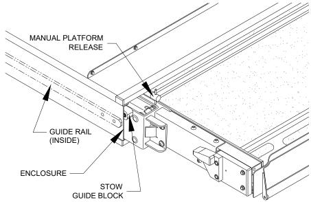
FIGURE 2-15: STOW GUIDE BLOCK ALIGNMENT
