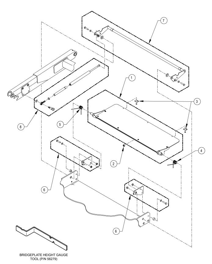
FIGURE 5-9: F9TF/F9TH BRIDGEPLATE ASSEMBLY
