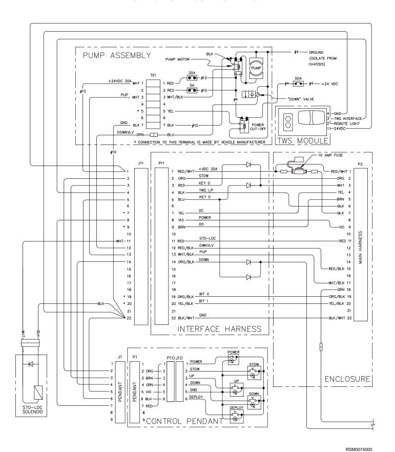
FIGURE 3-2: F9TF/F9TH DEDICATED ENTRY (W/O PULLBOX) ELECTRICAL DIAGRAM—SHEET 1 OF 3
