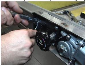
FIGURE 4-11: LOOSEN JAM-NUT
