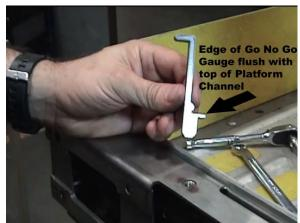
FIGURE 4-5: ROLLSTOP ADJUSTMENT TOOL P/N 55273
