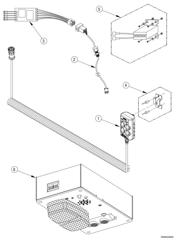
FIGURE 5-11: F9TF/F9TH-SERIES PENDANT, COUNTER & TWS ASSEMBLY
