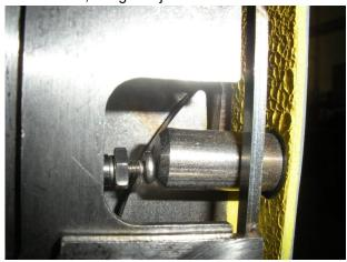
FIGURE 4-22: ROLLSTOP ACTUATOR
