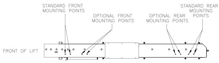
FIGURE 2: LIFT MOUNTING POINTS
