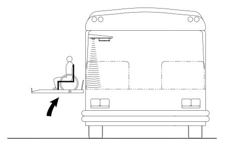
FIGURE 7: CHECKING NORMAL PLATFORM POSITION
