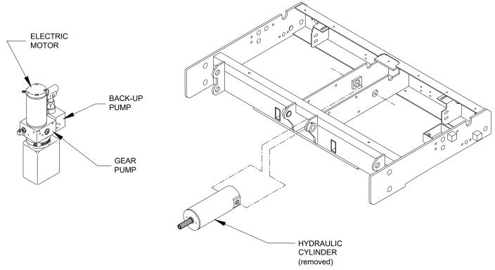
FIGURE 4-44: HYDRAULIC SYSTEM COMPONENTS
