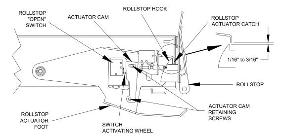
FIGURE 4-7: ROLLSTOP ACTUATION COMPONENTS
