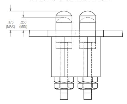
FIGURE 4-50: CONTACT SWITCH ADJUSTMENT
