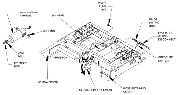
FIGURE 4-46: HYDRAULIC CYLINDER AND RELATED COMPONENTS
