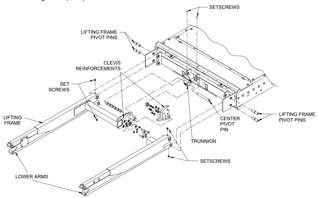
FIGURE 4-34: LIFTING FRAME COMPONENTS
