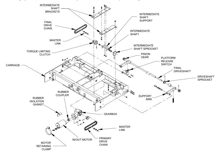
FIGURE 4-37: DEPLOYMENT SYSTEM COMPONENTS
