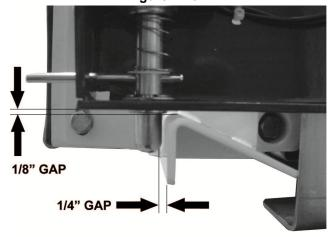
FIGURE 4-43A: STRIKER PLATE/STOW-LOCK ADJUSTMENT
