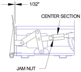
FIGURE 4-12: CLOSED ROLLSTOP ADJUSTMENT
