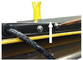
FIGURE 2-13. BRIDGEPLATE SWITCH RESET
