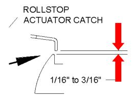
FIGURE 4-21: ROLLSTOP ACTUATOR
