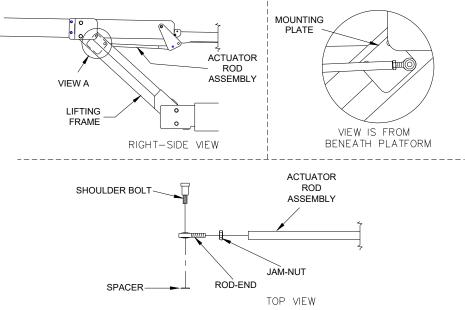
FIGURE 2-3: BRIDGEPLATE ACTUATOR ROD ASSEMBLY
