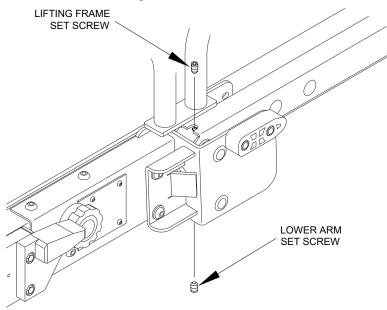
FIGURE 4-31: LIFTING FRAME AND LOWER ARM SET SCREWS
