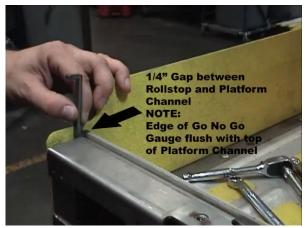
FIGURE 4-6: ROLLSTOP ADJUSTMENT TOOL (GAUGE)
