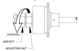
FIGURE 4-39: TORQUE LIMITING CLUTCH ADJUSTMENT
