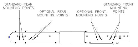
FIGURE 2-1: LIFT MOUNTING POINTS
