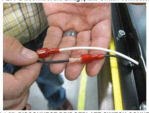
FIGURE 4-27. DISCONNECT BRIDGEPLATE SWITCH CONNECTORS
