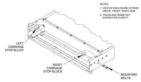
FIGURE 4-35: CARRIAGE STOP BLOCK LOCATIONS
