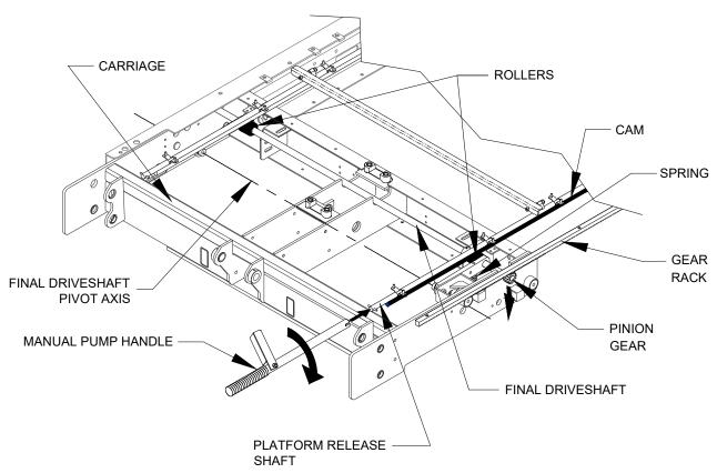
FIGURE 4-40: PLATFORM RELEASE COMPONENTS
