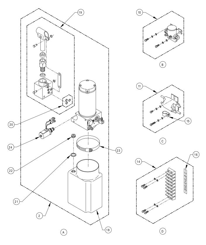
FIGURE 5-3: F9TF/F9TH-SERIES PUMP BOX ASSY (SHEET 2 OF 2)
