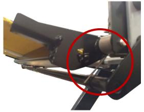
FIGURE 2-10. UNHOOK BRIDGEPLATE SPRING
