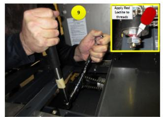
Once proper adjustment has been obtained, apply RED permanent Loctitie to threads and hold the inner nut with a wrench, and tighten the outside locknut with a torque wrench between 40 and 50 ft.lbs.
