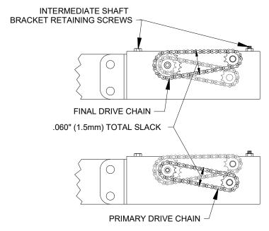
FIGURE 4-38: DRIVE CHAIN SLACK ADJUSTMENT
