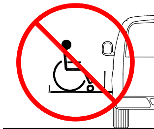
FIGURE 2-2: ALWAYS FACE OUTWARD WHEN RIDING ON THE LIFT PLATFORM
